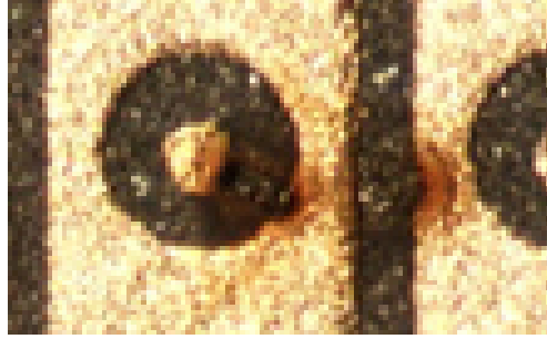
Figure 4.9: Microscopic photograph of a damaged electrode of \mu -PIC1.
