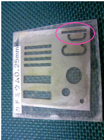
(a) Circled region was irradiated with a neutron beam.
