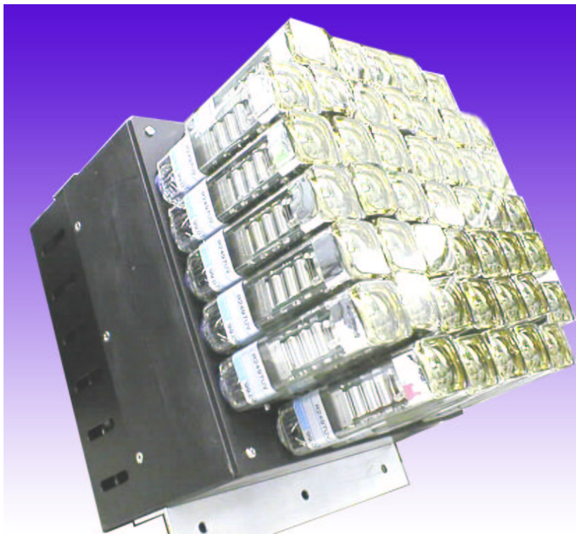
Figure 3.4: Photo Multiple Tube array which covers a field of view 0.75^\circ \times 0.75^\circ . The size of each PMT is 26\text{mm} \times 26\text{mm} (the photo-cathode is 23\text{mm} \times 23\text{mm} ). The black box behind PMTs is AMP-BOX which consists of amplifier chips (LeCroy TRA402S ).
